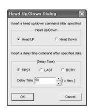
④ Set Head-Down at Point B using the same method. In LAST, set 200ms for time delay.
