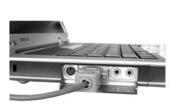
Serial port connection to the lap top (the location of serial port will differ depending on the PC).
